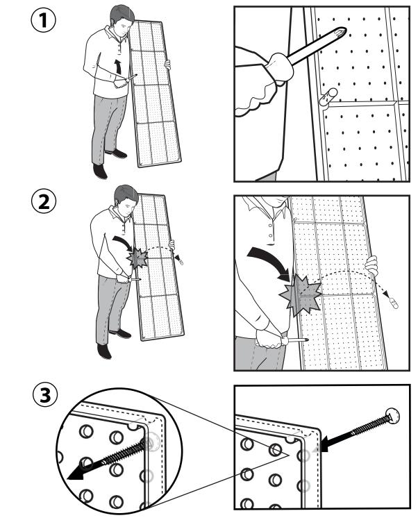
Use the pegboard holes as precut mounting holes.
